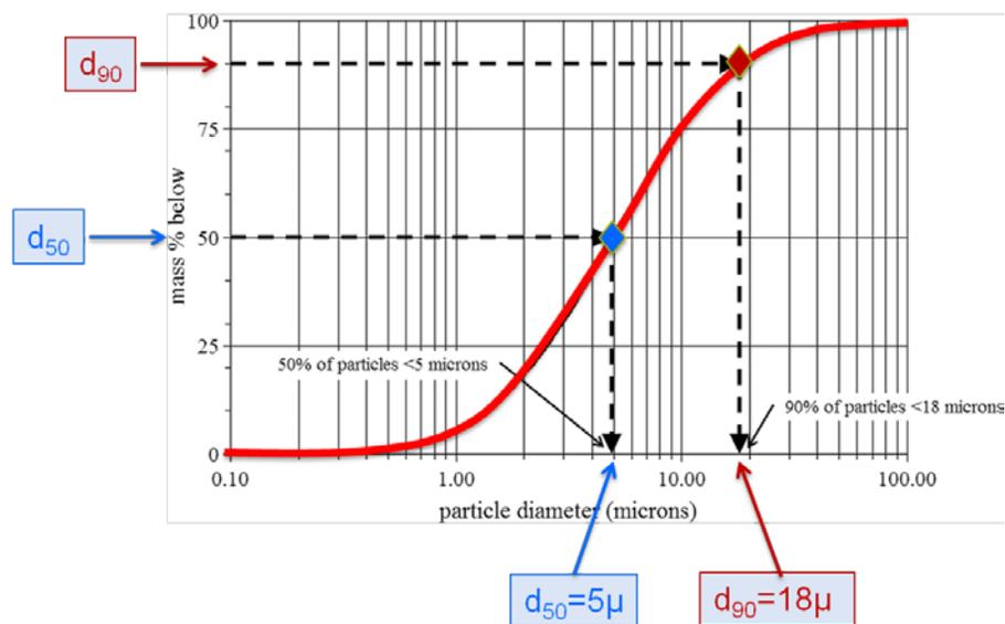
Figure 2. Example of a Particle Size Distribution graph for a  $d_{50}$ =50 microns.
